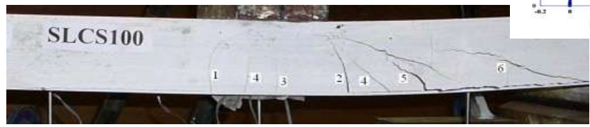
Typical crack pattern and sequence of appearance
