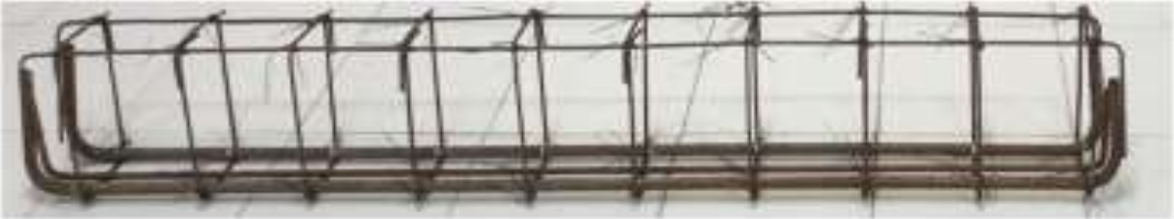
Stirrup Rebar As Transverse Reinforcement
