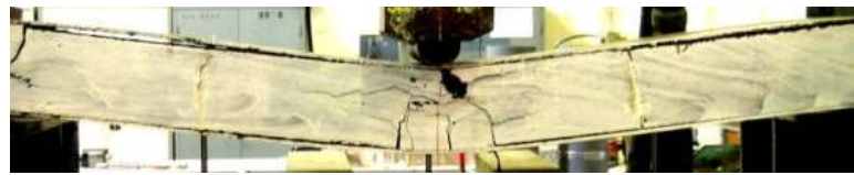
(e) Top plate buckling failure (beam SLCS)
