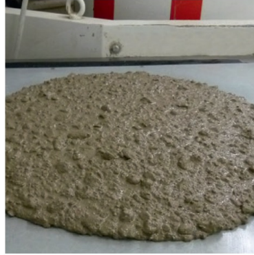
Concrete with fine aggregates contaminated with swelling clay, with MasterSuna SBS
