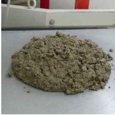
Master Builders Solution Concrete with fine aggregates contaminated with swelling clay, without MasterSuna SBS
