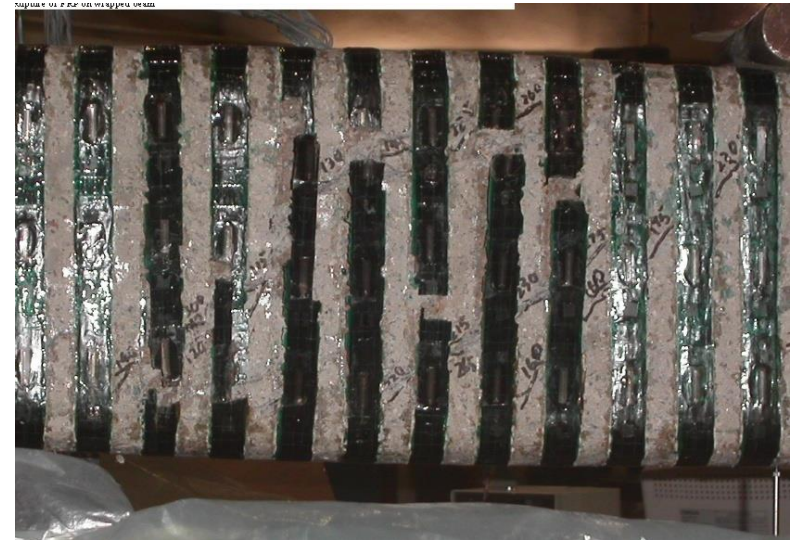
FRP rupture failure
