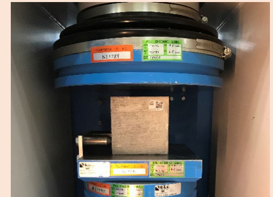
Placing samples onto compression test machine
