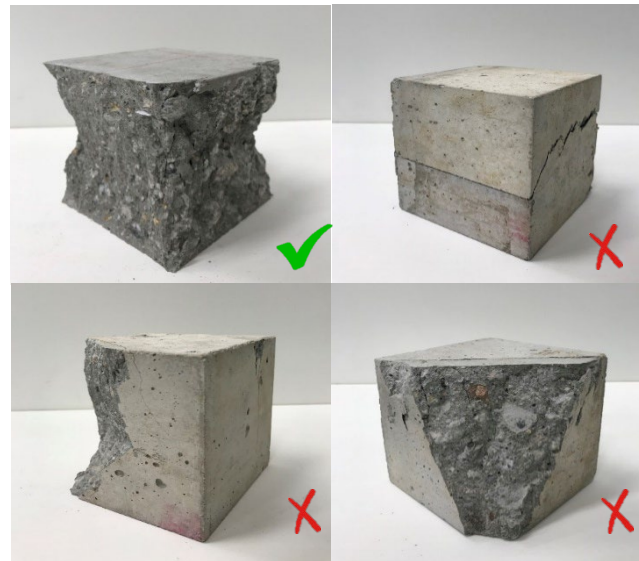
Identification of fracture pattern
