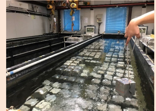
Placing test samples into curing tank
